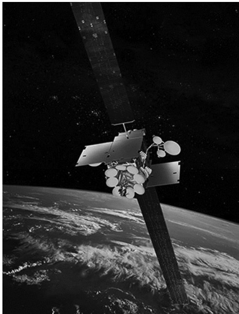
Figure 2. Inmarsat-5, a Boeing 702HP high throughput satellite
